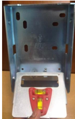
Figure 36: Leveling Jig Fixed to the Bracket
