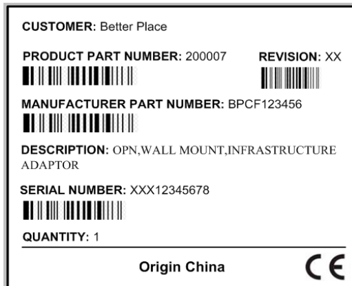
Figure 15: Double Socket Wall CS Infrastructure Package Label
