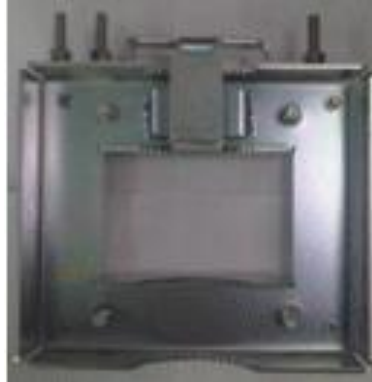
Figure 119: The Omega Pole Holders Removed
